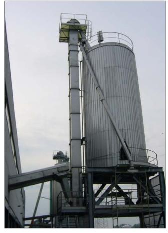
Each bucket elevator will be dimensioned from B.S.P. Engineering technical department according to the physical characteristics of the product.
