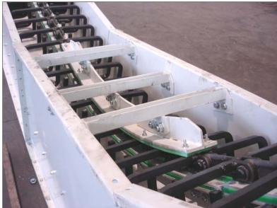
The employ of high resistance steel for the construction of the casings and of the guides of chains assures this type of chain conveyors as particularly suitable for the conveying of abrasive and corrosive bulk products.
