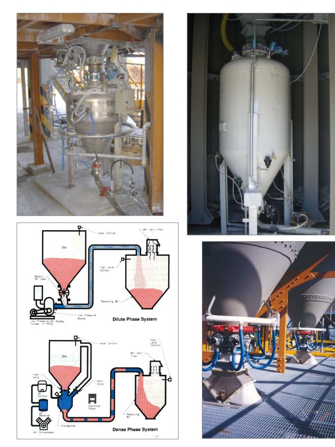
Each pneumatic conveying system in dense phase will be dimensioned from B.S.P. Engineering technical department according to the physical characteristics of the product.
