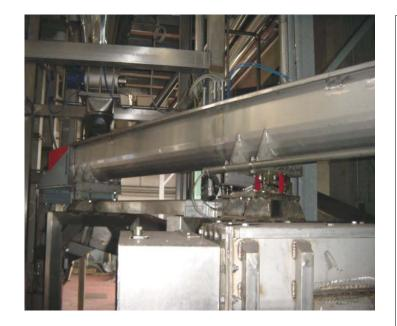
The screw conveyors, baggers, weighers realized by B.S.P. Engineering are made of galvanised steel, painted and stainless steel.
