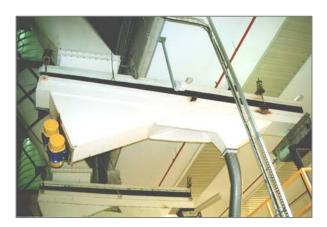
Each vibrating conveyor will be dimensioned from B.S.P. Engineering technical department according to the physical characteristics of the product.
