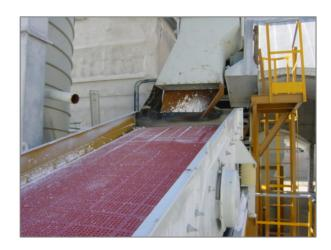
B.S.P. Engineering conveyors, feeders and extractors are specially suitable for high temperature, high density and abrasive products.
