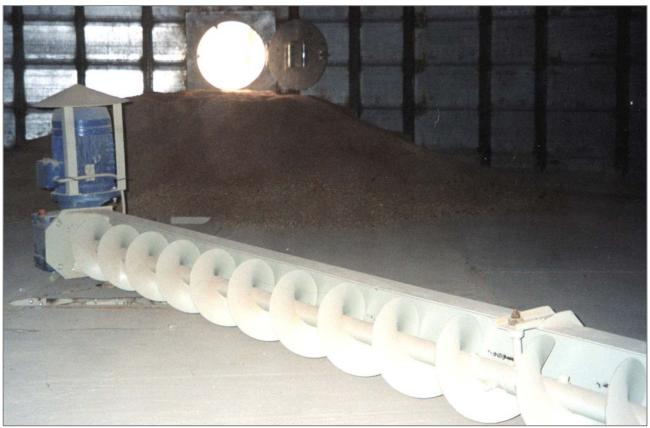
Each Rotating Screw Extractor is dimensioned from B.S.P. Engineering technical department according to the physical characteristics of the product, to the silo size and to the requested capacity.
