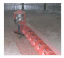
Rotating screw extractor for flat bottom silos with diameter up to 18 meters. The screw, open on one side and covered on the other side, by rotating on the flat bottom of the silo, allows the discharging of the residual cone.
