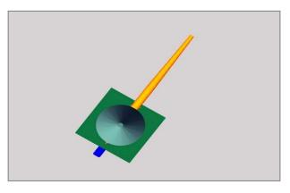
A cover deflector fixed on a idle large diameter anti friction bearing anchored on the top of the rotating steel frame, allows to the same frame to rotate without the stress due to the exiting over load inside the silo full of product.
